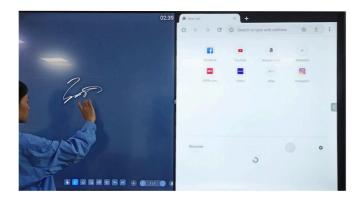
After the dual-screen display is turned on, a currently running application is displayed on the left and right, which can be operated independently
